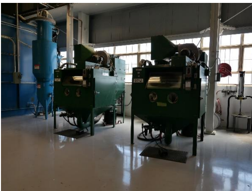
Photograph #5: Two blast booths for steel and aluminum aluminum parts.
