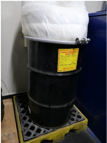
Photograph #9 – 35-gallon container of paint washer filter.
