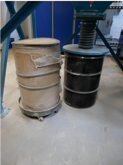
Photograph #3 – Unmarked black 55-gallon container of blast media and dust in the baghouse room.
