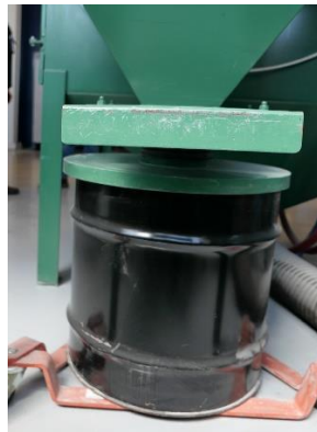
Photograph #6: Unmarked 30-gallon container to collect paint/blasting media chips.
