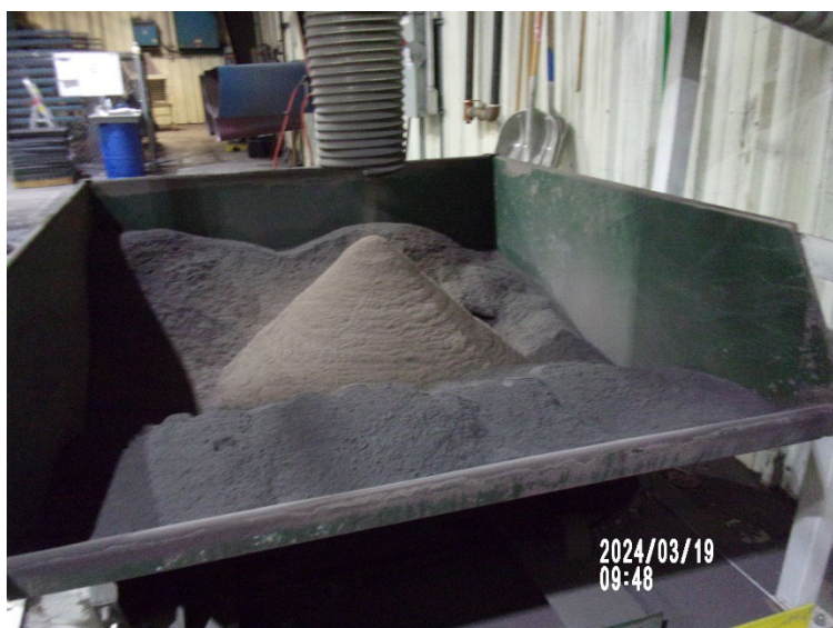
Photograph 3: Materials from the air pollution control baghouses that will be reinserted into the production process.
