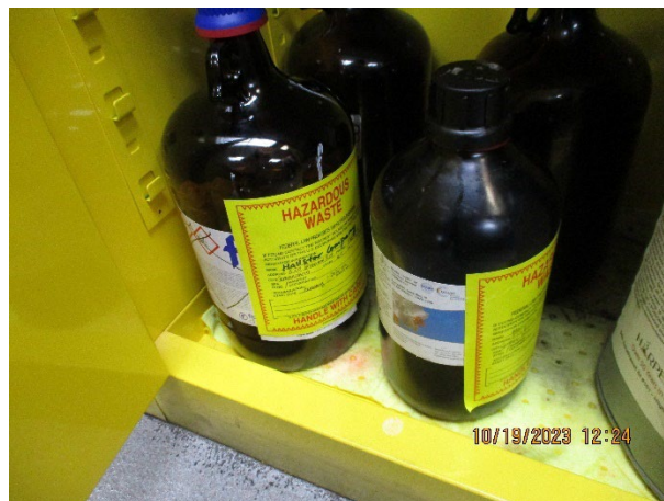
Photo 2: Hazardous waste labels placed on SAA containers in laboratory.
