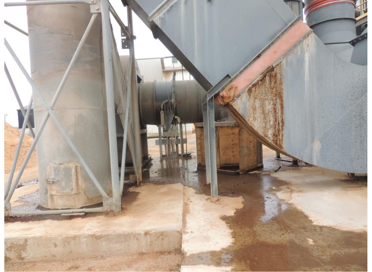
DSCN4060 – Dust collector/baghouse off of hammer mill
