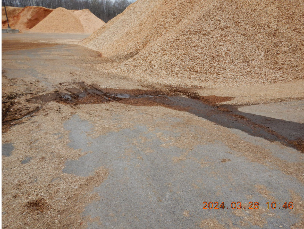
DSCN2749 - Condensate runoff from manufacturing process
