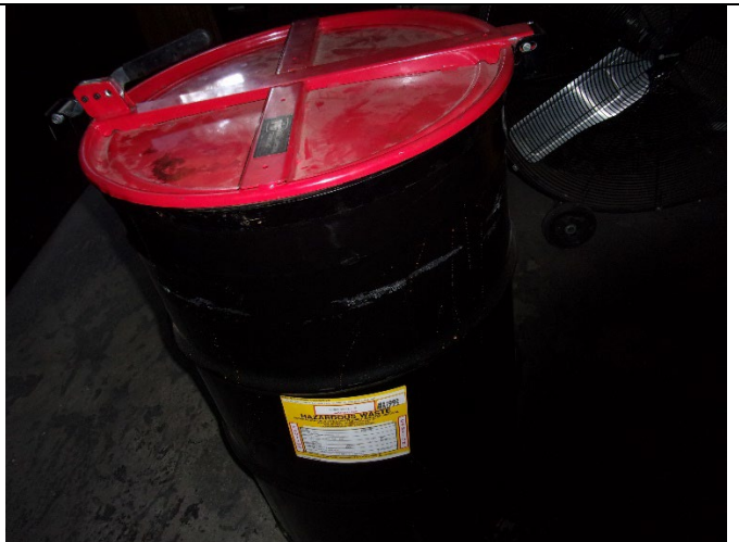
Figure 2: 9:38 AM West Drum Storage Room One 55-gallon container with hazardous waste label, and indication of the hazards of the contents.
