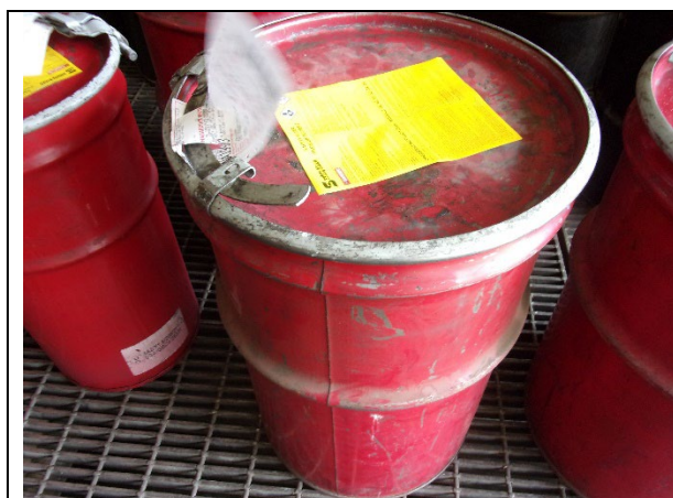
Figure 7: 9:57 AM Return and Fill Station One 35-gallon container with hazardous waste label, and indication of the hazards of the contents.
