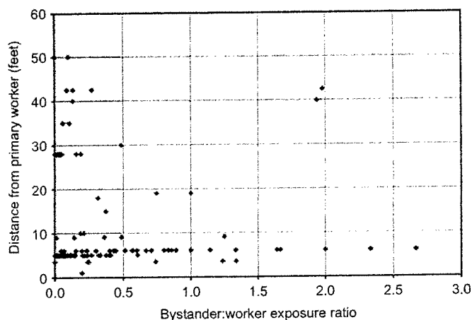
Figure 4. X-Y scatter plot for published data. bystander:worker ratios of airborne asbestos concentrations at distance from a source
