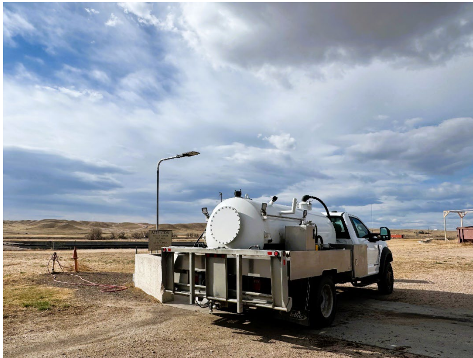
Figure 9 – Dry Creek POTW Septic Disposal Station – Septic Truck Discharge
