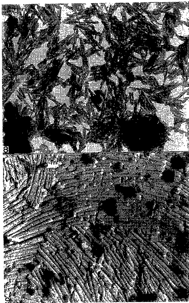
Fig. 8. Electron micrograph of chrysotile from fragments of massive serpentinite in the Coalinga asbestos deposit (248-43-4). Magnification = 19,500 \times .
