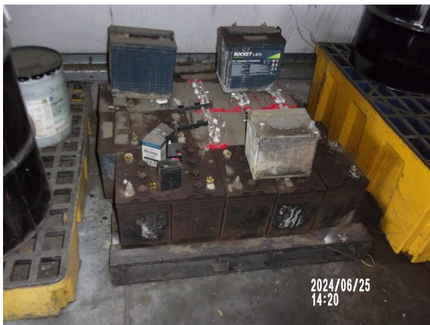
Photograph 13: Pallet of unlabeled and undated universal waste batteries.
