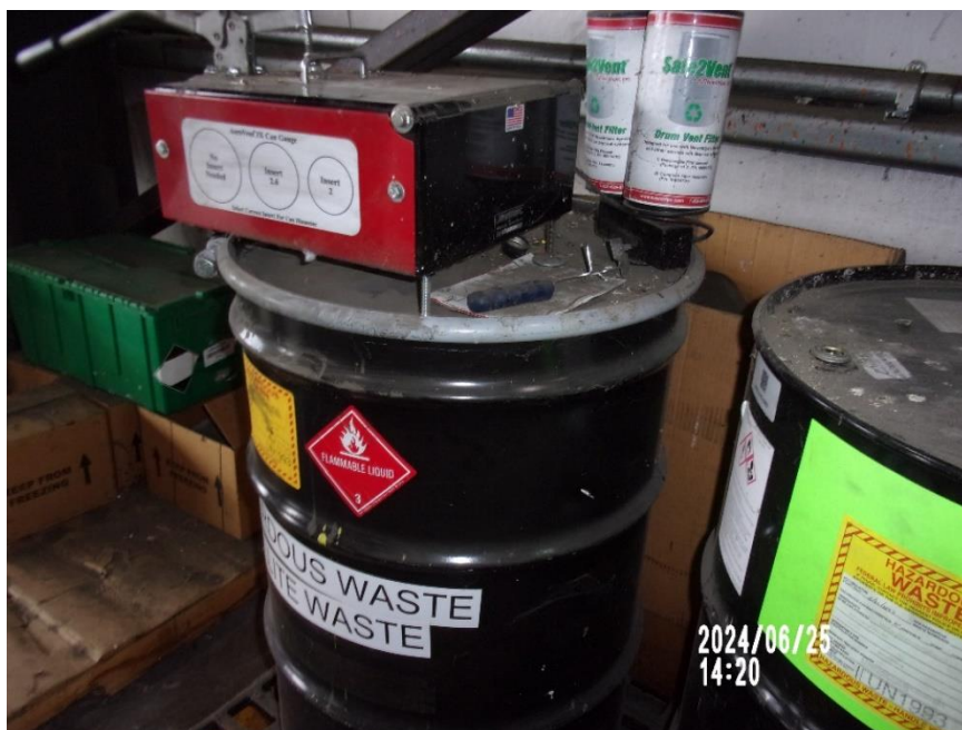
Photograph 12: Aerosol can puncturing device over a HW SAA container.
