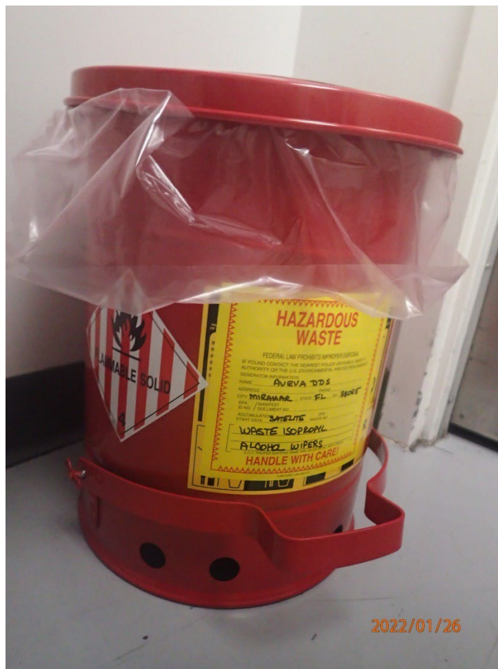
Photo 1: The SAA contained one (1) 5-gallon closed container labeled “Hazardous Waste—Waste Isopropyl Alcohol Wipers”. The container was also marked with an indication of hazard for flammable solid.
