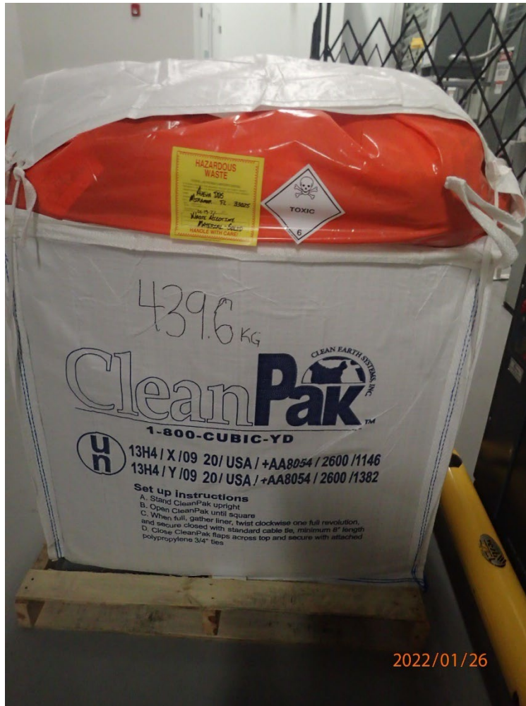
Photo 8: One (1) CYB with a liner that was full and with a marked weight of 439.6 kg. The CYB was tied closed on a pallet ready for shipment offsite. The CYB was labeled “Hazardous Waste—Waste Nicotine Material Solid” and dated 01/19/2022. The CYB also had a DOT Toxic placard displayed as an indication of hazard.
