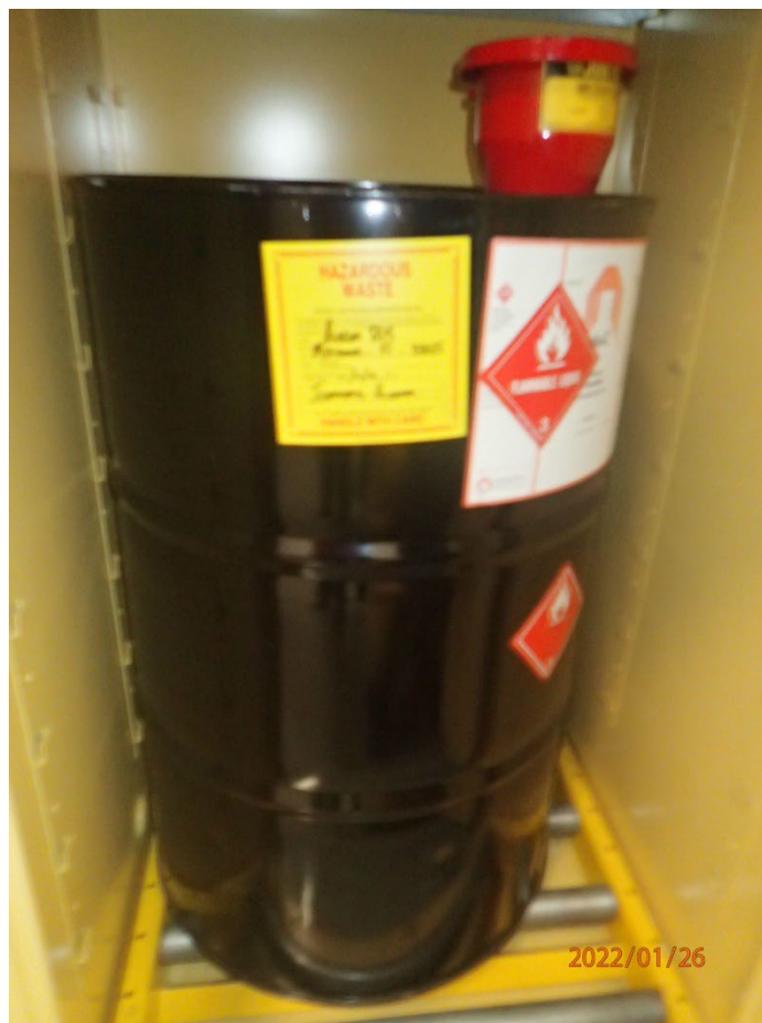
Photo 4: One (1) 55-gallon closed drum labeled “Hazardous Waste—Isopropyl Alcohol”, dated 11/12/2021. The drum had a DOT flammable liquids placard to indicate the hazard.
