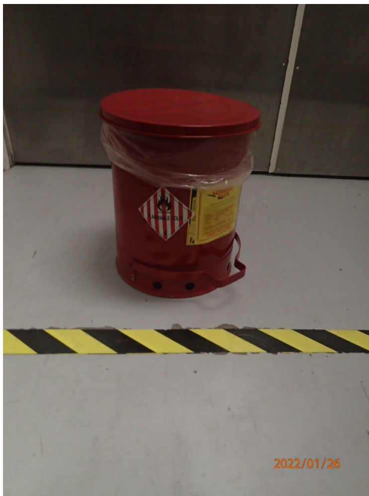
Photo 9: SAA for Delta Packaging and Secondary packaging contained one (1) 5-gallon closed container labeled “Hazardous Waste—Waste Isopropyl Alcohol Wipers”. The container was also marked with an indication of hazard for flammable solid.
