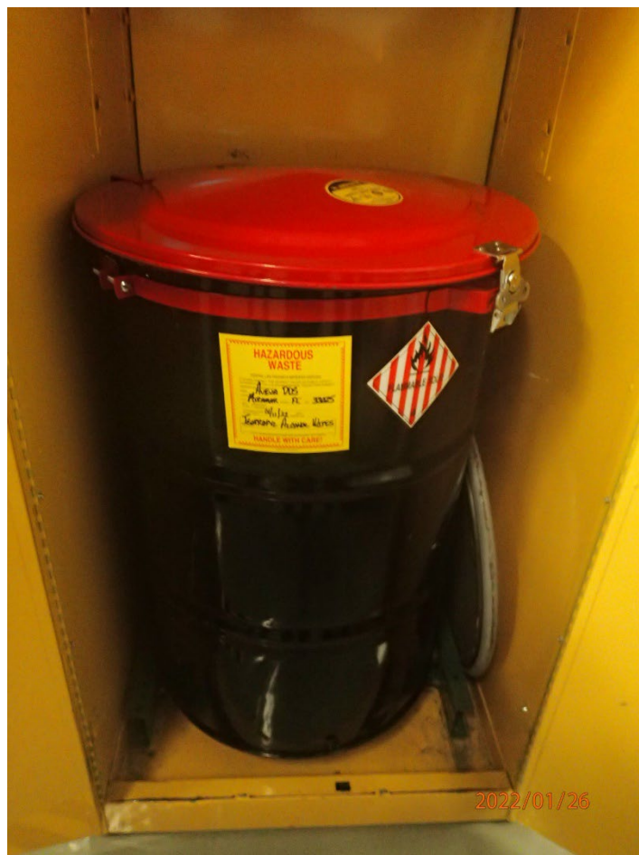
Photo 3: One (1) 55-gallon closed drum labeled “Hazardous Waste—Isopropyl Alcohol Wipes”, dated 01/11/2022. The drum had a DOT flammable solids placard to indicate the hazard.
