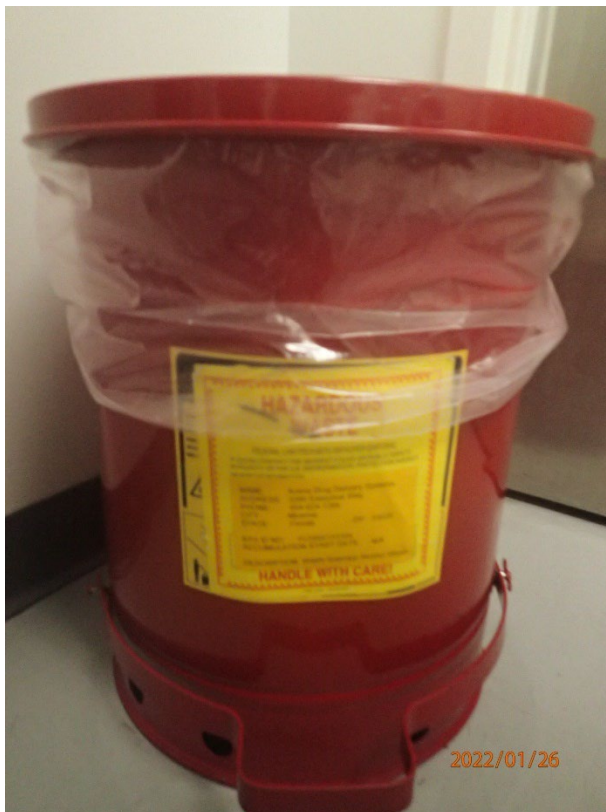
Photo 2: The SAA contained one (1) 5-gallon closed container labeled “Hazardous Waste—Waste Isopropyl Alcohol Wipers”. The container was missing an indication of hazard. This was corrected onsite.
