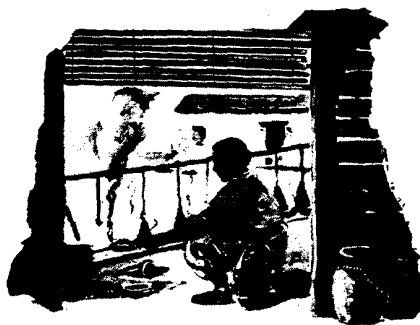
Primitive method of producing Lamp Black with smoking lamps.
