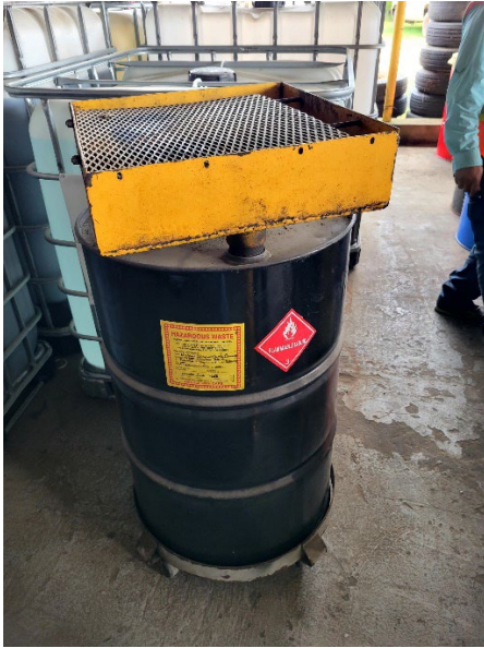
Photo #5 – Maintenance Area – open flammable hazardous waste container.
