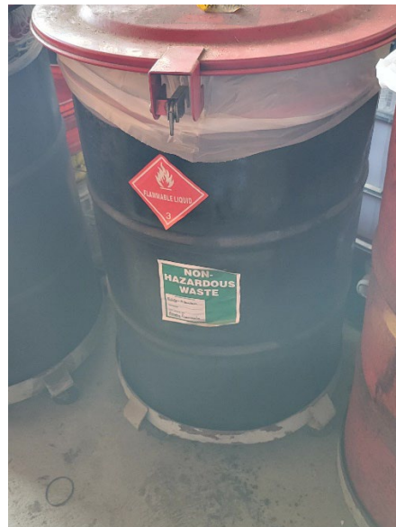
Photo #8 – 55-gallon container of used oil filters mislabeled.
