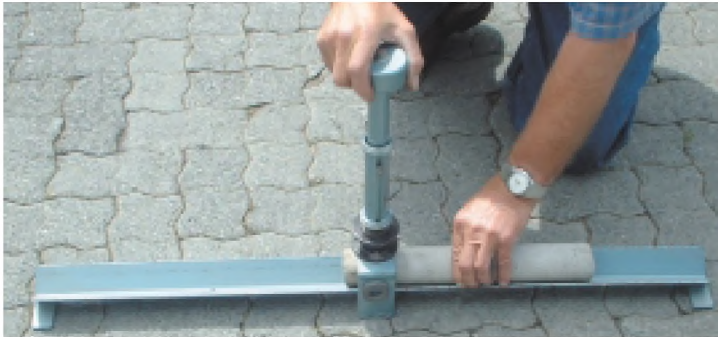
Impact splitting was found to be effective for South African conditions.
