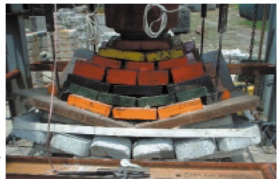
Result of a static load of around 40 tons.
