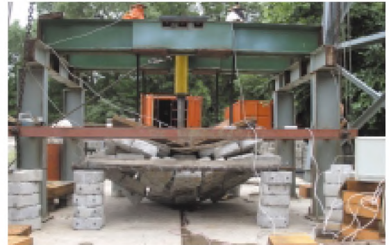
Result of an impact from a mass of 3 tons travelling at a speed of 5 m/s (37,5 kJ).
