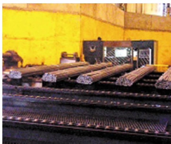
Top: Rotary forging of smartbolt ingot. Bottom: Batches of smartbolt wire rod (20 mm in diameter).
