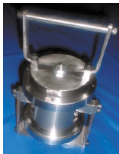
A heavy tungsten slug was used to reduce the size of the absorber shown above while still tuning it by changing the pressure in an air spring.
