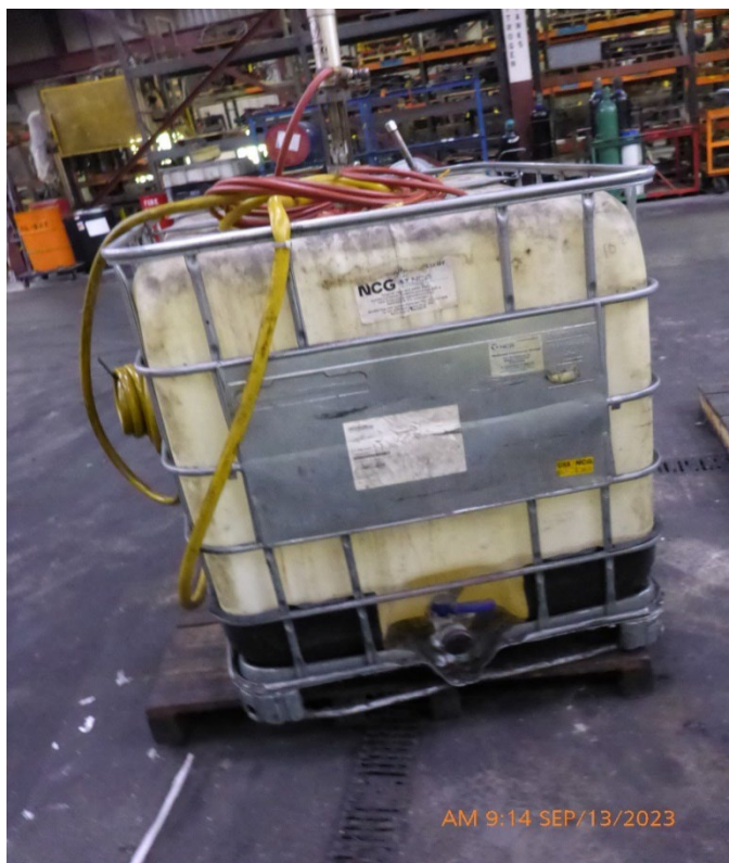
Photograph 3: Chemical tote stored directly over trench drain at PHB.
