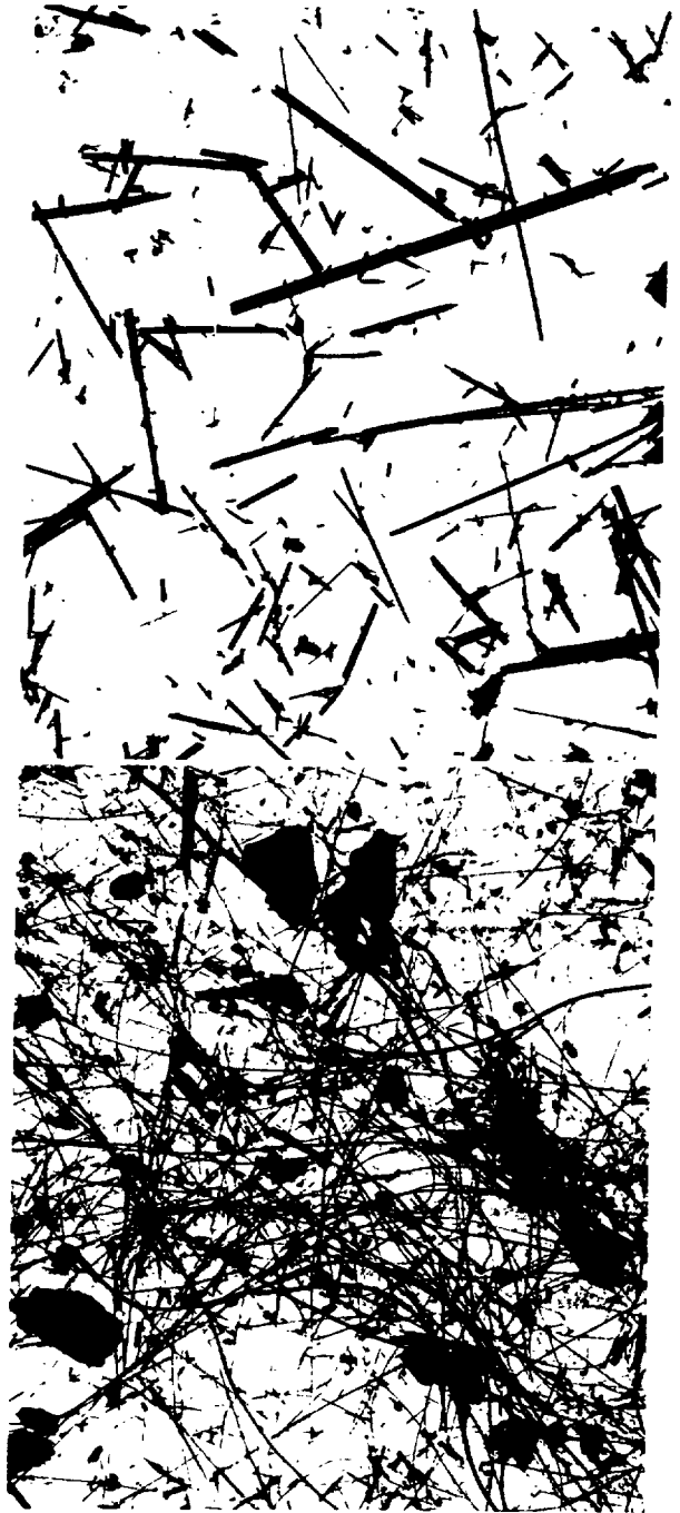
FIG. 1.—Electronmicrograph of SFA chrysotile ( \times 1875 ).
