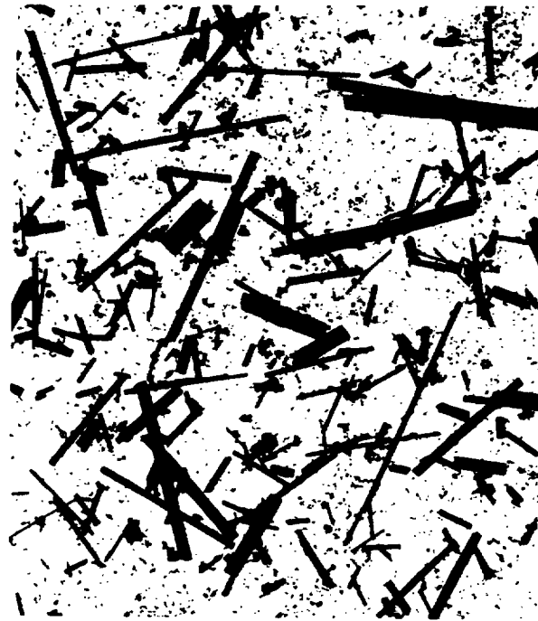
FIG. 4.—Electronmicrograph of UICC amosite ( \times 1875 ). 10 \mu m
