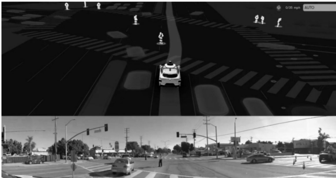
A Waymo vehicle recognizes and adheres to a police officer directing traffic at a Los Angeles intersection. 23
