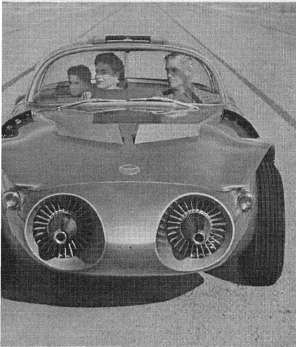
Strength and light weight open automotive field to titanium metal. General Motors' new experimental gas turbine-powered car, the Firebird II, sports an all-titanium body.
