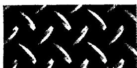
Relative size of projections on Large, Small and Light Patterns of Inland 4-Way Floor Plate. Projections are respectively 1 1/2", 1", and 3/4" long.
