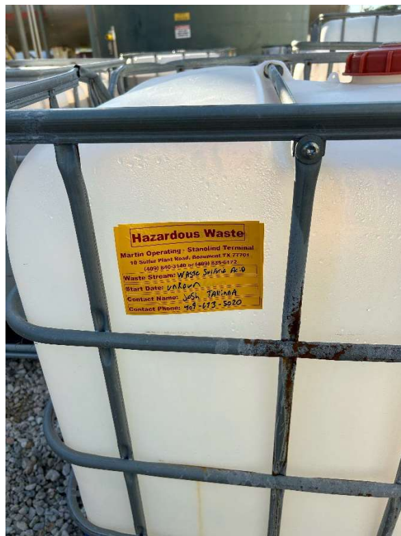
Hazardous Waste Sticker Affixed to Tote
