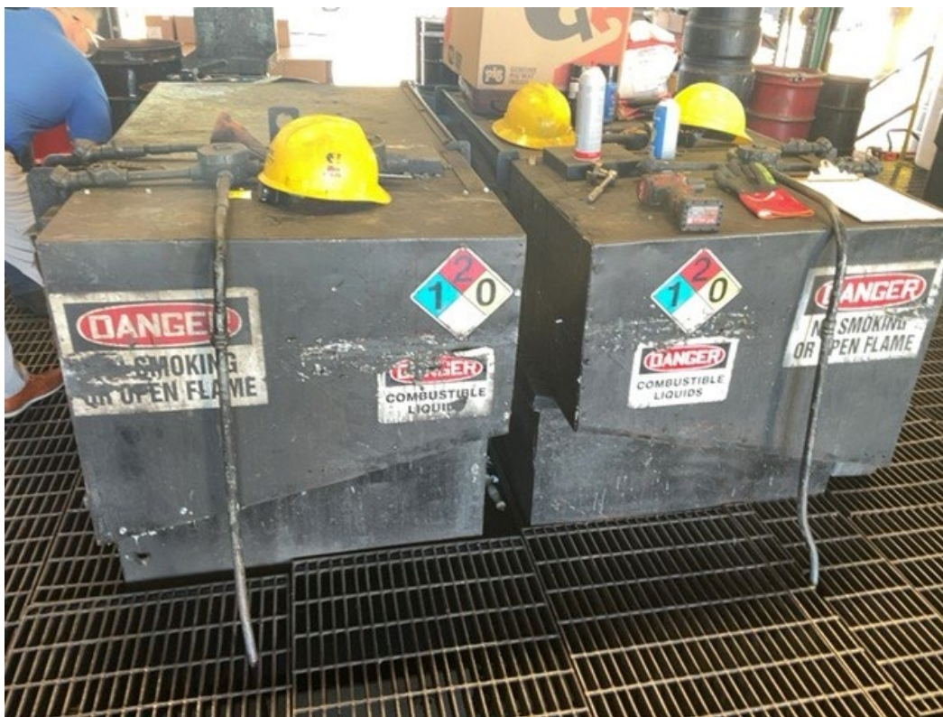
Photo 1 – Labeling on Wet Dumpsters in the return and fill area
