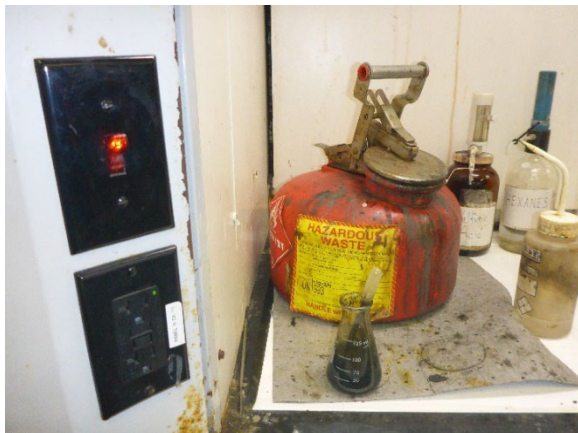
Photo 2: One of two 2.5-gallon containers in the laboratory SAA for accumulating waste flammable liquids generated in the laboratory. This container was observed in Laboratory Hood #2.
