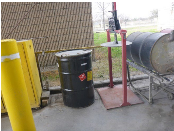
Photo 9: Compactor unit used to compact hazardous waste solids into 55-gallon containers in Area 6100.
