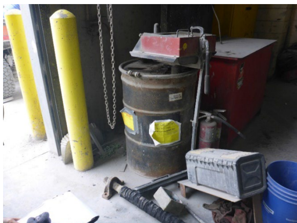
Photo 20: 55-gallon container with an aerosol can puncture device in the Holcim Maintenance SAA for accumulating the contents of waste aerosol cans.
