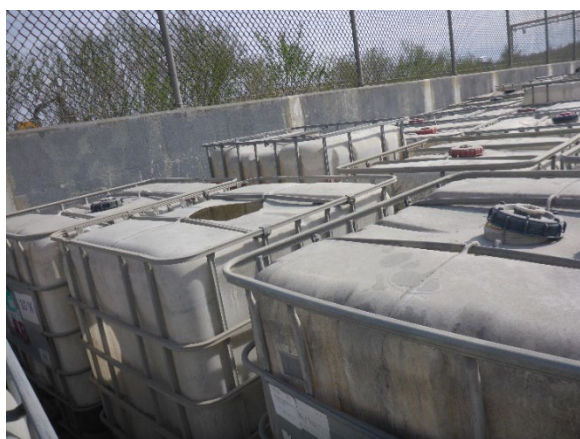
Photo 15: Open tote among the approximately fifty 275-gallon totes in the area identified for a future tank farm.
