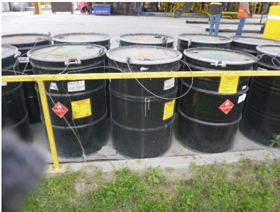
Photo 8: Some of approximately twenty-five 55-gallon containers of hazardous waste compacted solids in Area 6100. One container, dated November 22, 2023, was not marked with an indication of the hazards of its contents.
