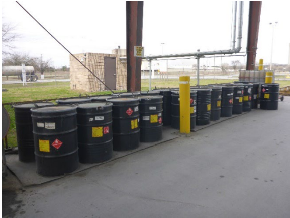
Photo 7: Approximately twenty-five 55-gallon containers of compacted hazardous waste solids in Area 6100.
