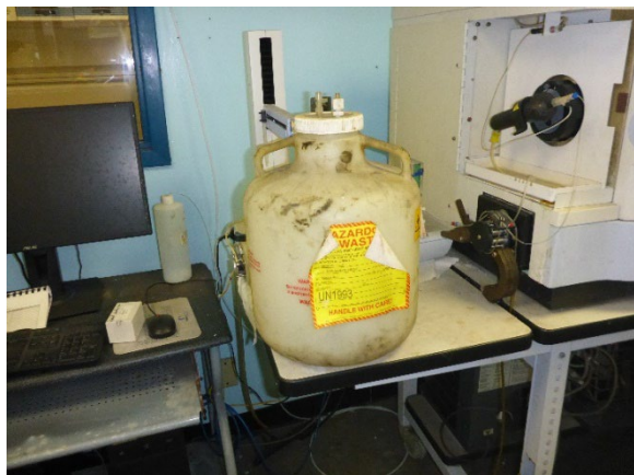
Photo 4: One of two 5-gallon containers of waste nitric acid in the laboratory SAA. This container was connected to an ICP testing unit.
