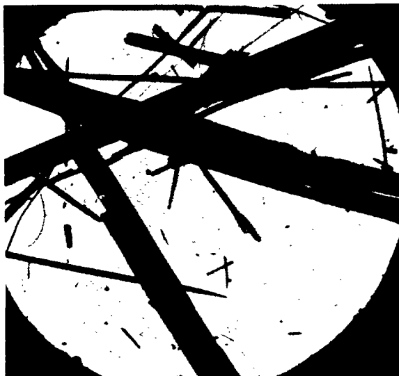
Figure 12.—Electron micrograph, tremolite asbestos. x 1,733.
