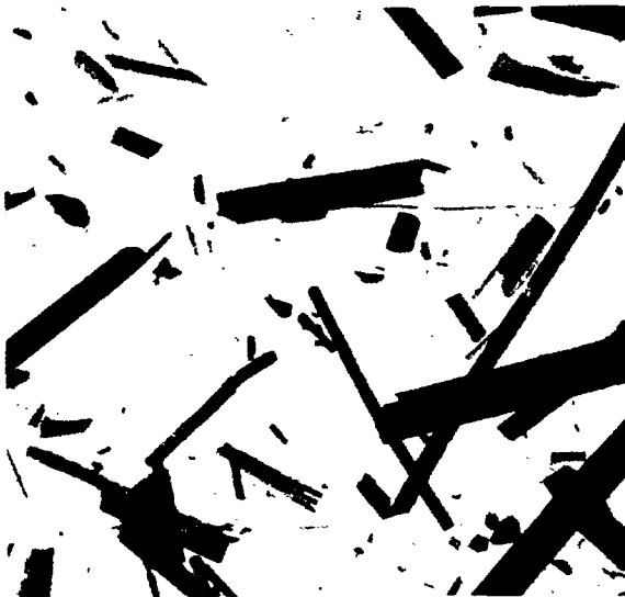
Figure 5.—Electron micrograph, amosite asbestos. x 15,200.
