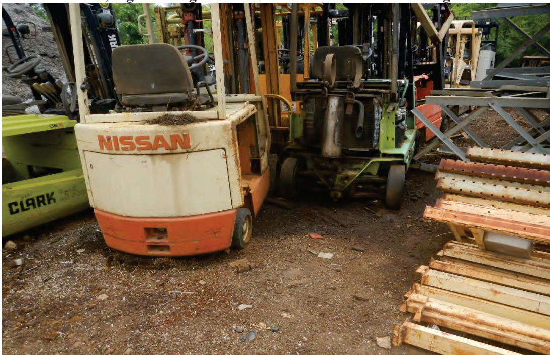
Photo 1, Significant ground discoloration around the salvaged forklifts
