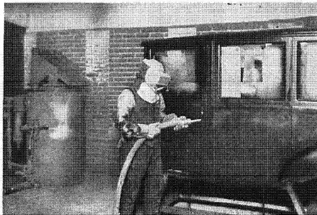
The old finish is removed from the body by sand blasting, which is the surest and quickest way
