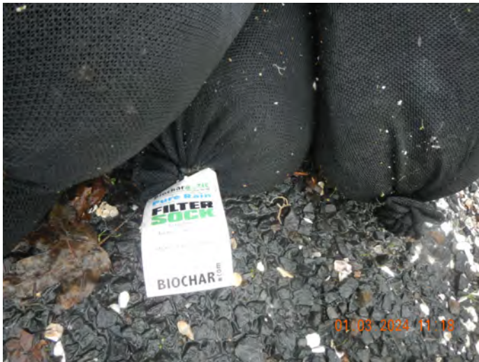
Photo #:35 (DSCN3484) Description: Photo of Biochar filter socks, stored near Pond 2.
