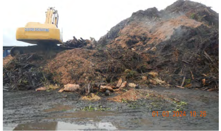
Photo #:06 (DSCN3455) Description: Photo of wood debris storage/processing area. The wood product is brought in from Recology and processed on-site as hog fuel and hauled daily to a paper mill in Wauna, WA.
