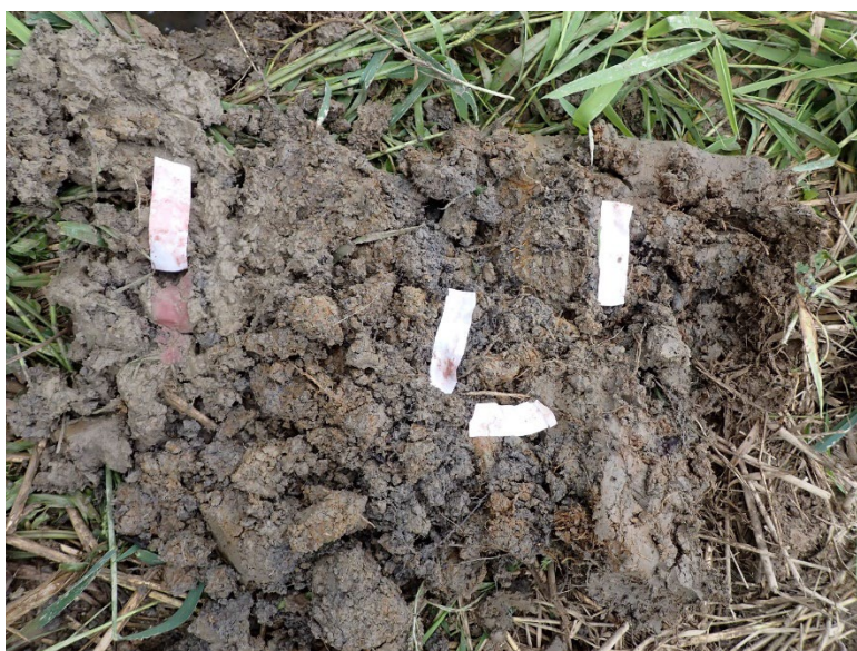
Photograph VIII.L. DP3: Dipyrityl paper strips indicating the presence of iron in soil profile.
