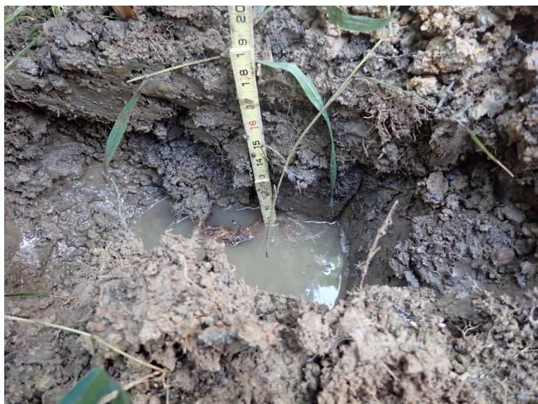
Photograph VI.I. DP2: High water table observed in soil profile location.
