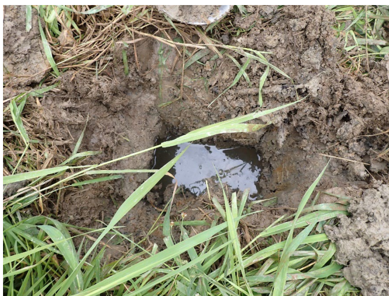
Photograph VIII.N. DP3: High water table observed in soil sampling location.
