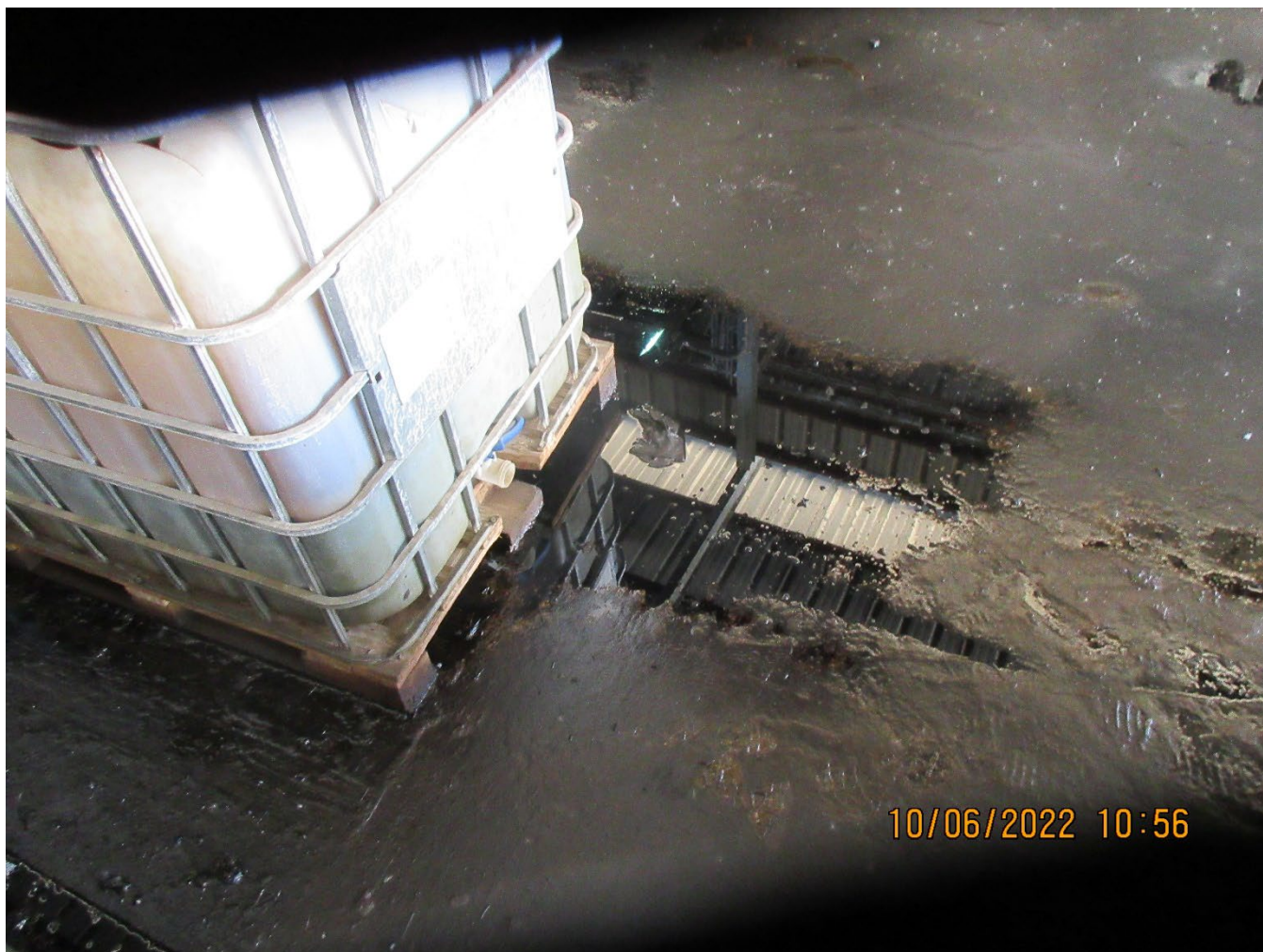
Photo 9 – Floor with used oil release in collection area
