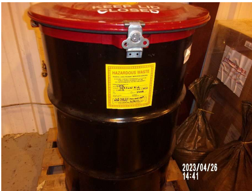
Photograph 38: SAA Container Missing Hazard Indicator
