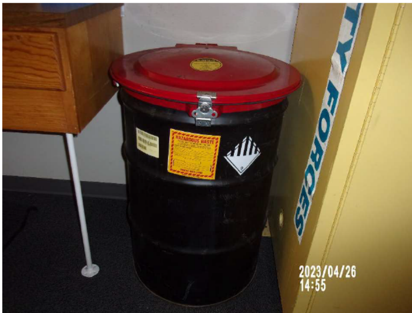
Photograph 39: Building 926 SAA Container, Missing Full Hazard Indicator Information
