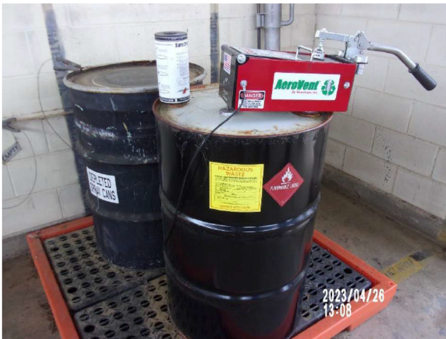
Photograph 33: Building 212, Aerosol Can Puncture Unit Over SAA Container
