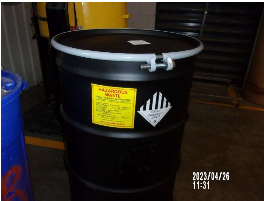
Photograph 8: Hazard indicator information added to container.
