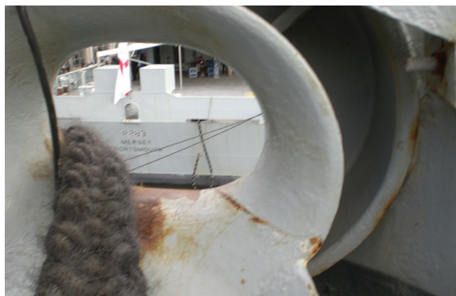
Figure 8. Steel Vessel Fairlead with Rusty and Worn Paint Surface
