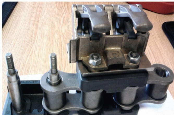
Figure 3. PEK 30 in Chain Element of Film Stretching Machine
