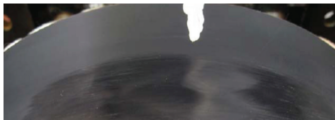
Figure 12. Effect of Extreme 'Stick/Slip' between PET Rope and Unlubricated Nylon Polymer Fairlead Section, 'Loud Bangs' with Each Slip. The Pattern of the PET Rope is Impressed into Sheave, 'Dry' Friction Coefficient of 0.36
