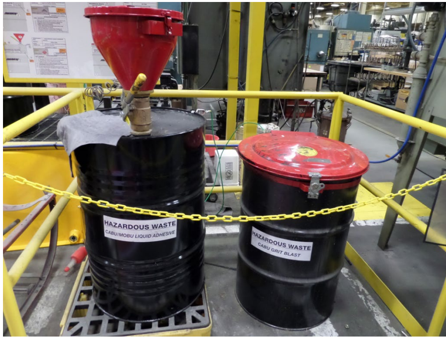
Photograph 5: SAAs for spent alcohol (D001) from cleaning activities and spent blast media (D008) from surface preparation activities. The containers were neither marked nor labeled with an indication of the hazards of their contents.
