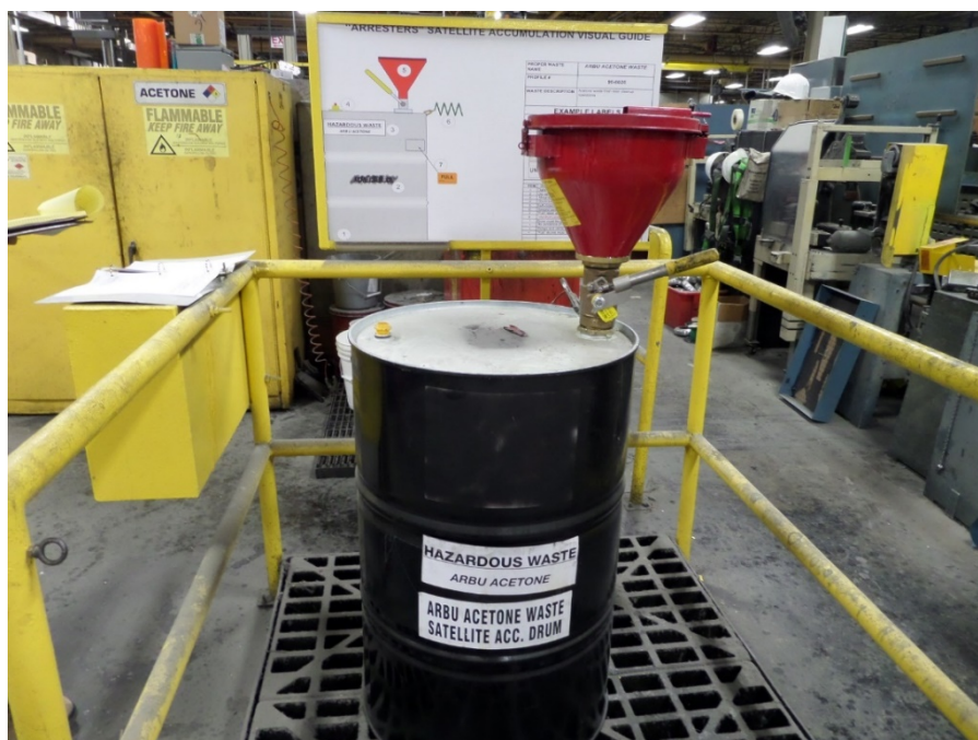
Photograph 1: Spent acetone (F003/D001) 55-gallon accumulation container at a satellite accumulation area (SAA) in the Arrester Business Unit (ARBU). The container was neither marked nor labeled with an indication of the hazards of its contents.
