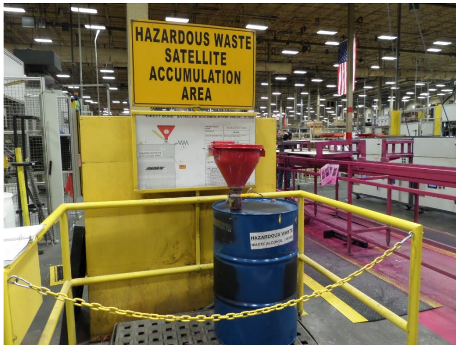
Photograph 3: Spent alcohol (D001) 55-gallon container from cleaning activities conducted in the Molding Business Unit. The container was neither marked nor labeled with an indication of the hazards of its contents.
