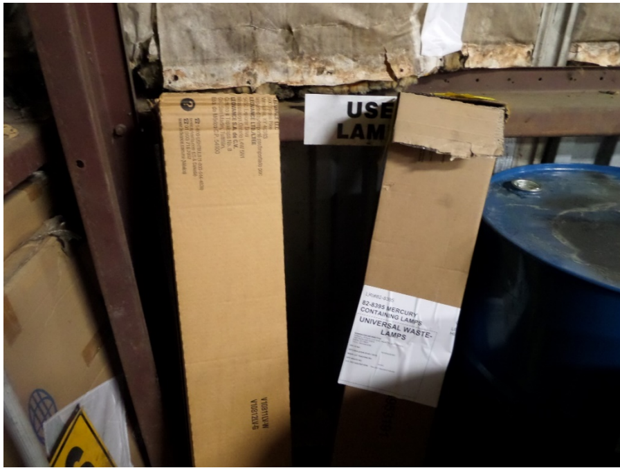
Picture 11: Universal waste lamp containers in the facility's hazardous waste CCA. Neither box was dated. One box was neither marked nor labeled "Universal Waste - Lamp(s)," or "Waste Lamp(s)," or "Used Lamp(s)."
