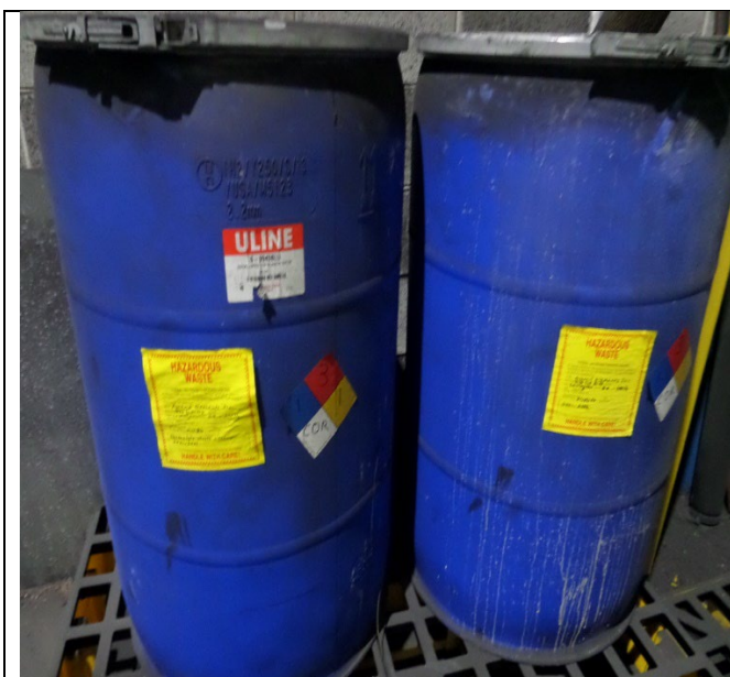
AEI. Central Accumulation Area (CAA). The inspectors observed the CAA was storing ignitable hazardous waste and not identified with the words "no smoking" Photograph 7 taken at 12:13 p.m.
