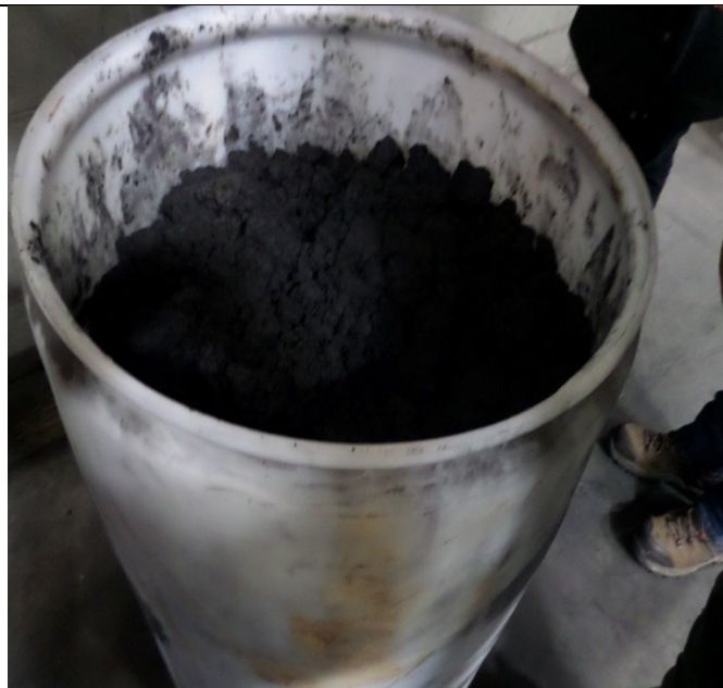
AEI. AEI. Container of Black Mass Near Wastewater Treatment System. The inspectors observed a 55-gallon container with a small hole in the container's top near the wastewater treatment system. AEI representatives opened it and indicated the contents was black mass was sent from AEI's Westboro, Massachusetts research and development program. Photograph 13 taken at 12:32 p.m.
