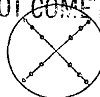
Figure 1-4. Cross section of circular stack showing location of traverse points on perpendicular diameters.
