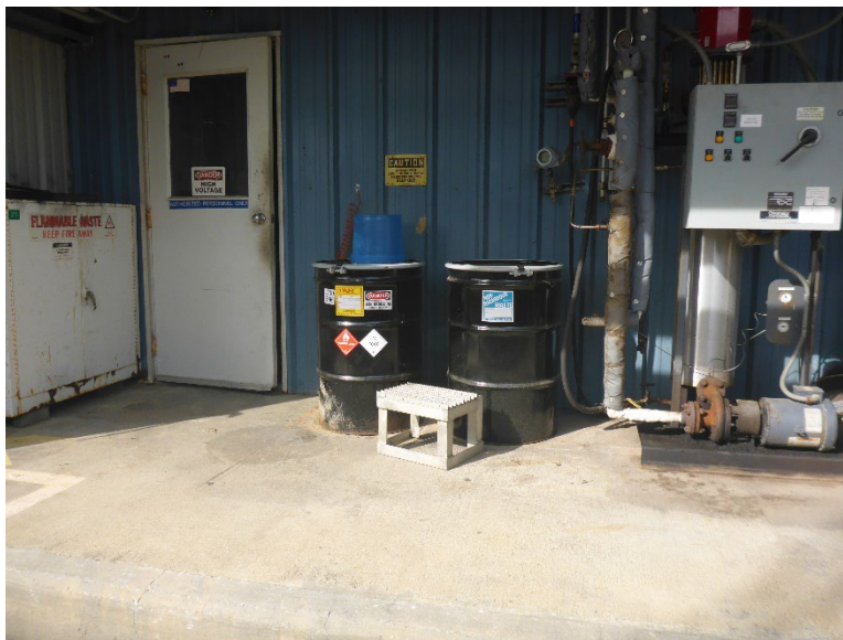
Photo 9: One 55-gallon drum, which was labeled hazardous waste (acrylonitrile, styrene) and identified as flammable and toxic, in the first Pilot Plant SW End SAA.
