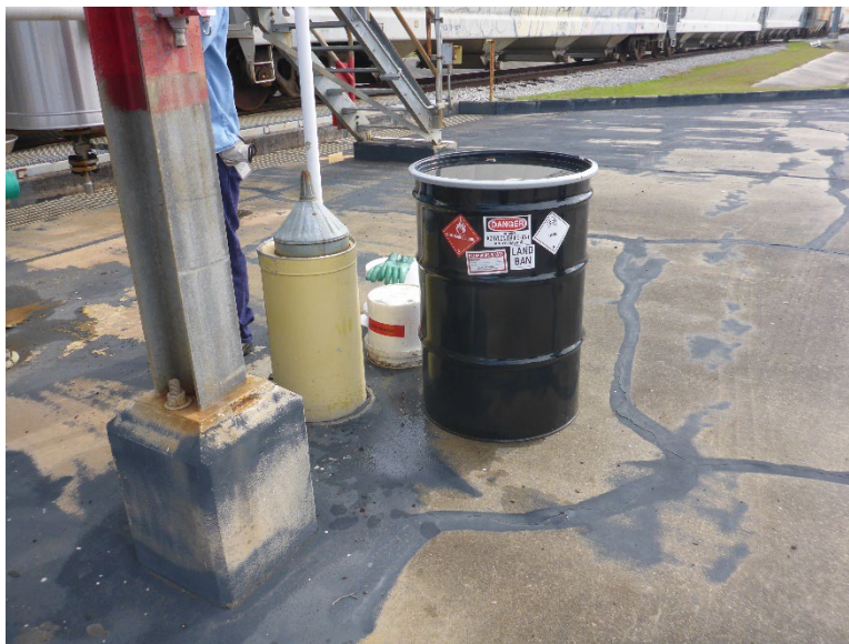
Photo 7: One 55-gallon drum, which was labeled hazardous waste acrylonitrile (AN) and marked to indicate that the contents are flammable and toxic, in the Truck Unloading SAA.
