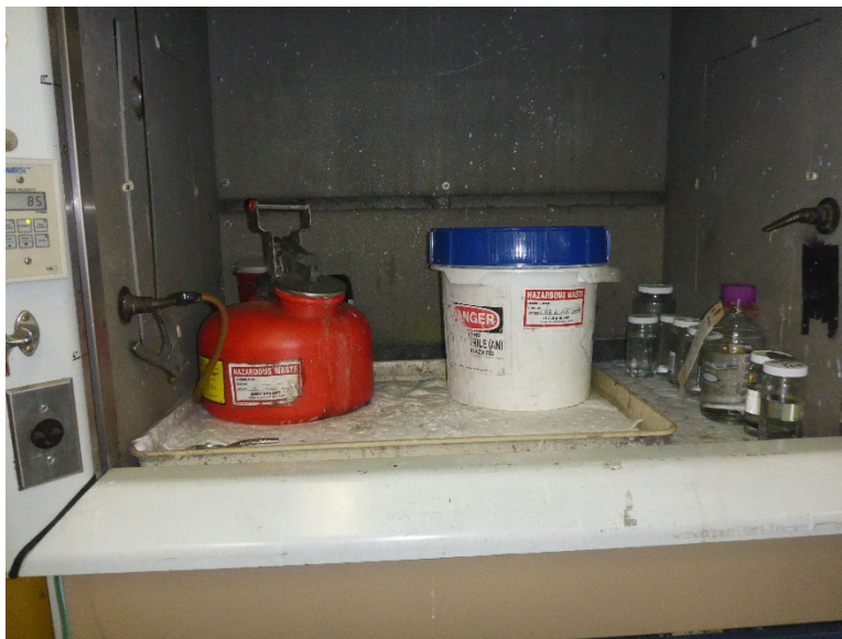
Photo 12: One flammable can and one 5-gallon bucket in the Laboratory SAA. Each container was labeled with the words “hazardous waste,” but neither was marked with an indication of the hazards of its contents.
