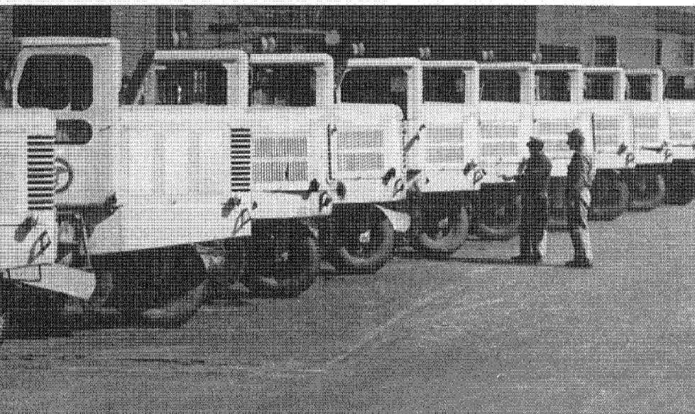
Armies of motorized brooms help New York clean 800,000 curb miles of street per year. Under each machine is long-wearing broom of nylon filament.
