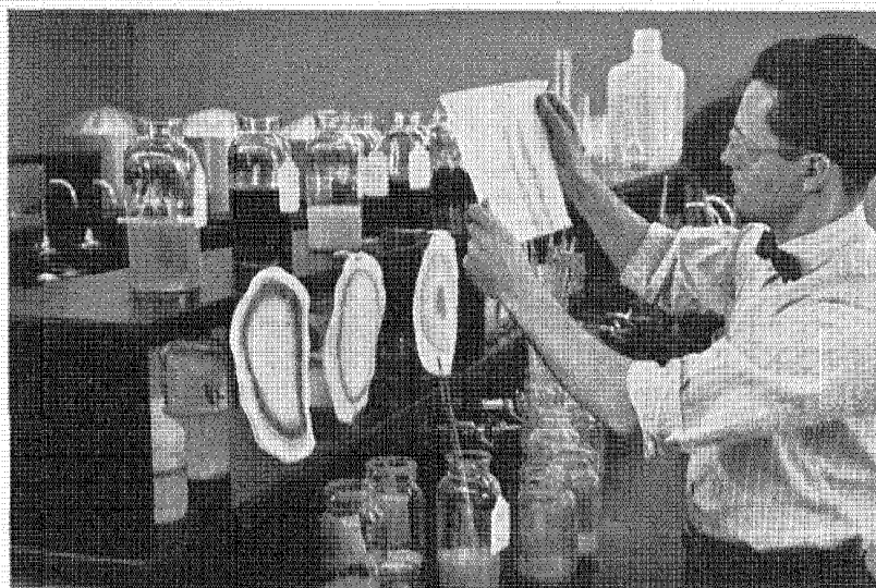
In modernized leather lab, colorist James Loper spots a dye solution to find strength relationships before making a sample dyeing.
