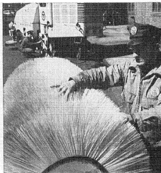
Armies of motorized brooms help New York clean 800,000 curb miles of street per year. Under each machine is long-wearing broom of nylon filament.
