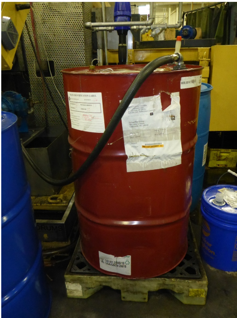
Photo 4: 55-gallon red metal drum in the Finger Follower Heat Treat Process Area. The drum is used to accumulate used oil pumped from the bottom of the Safed #6 De-Oiler machine.
