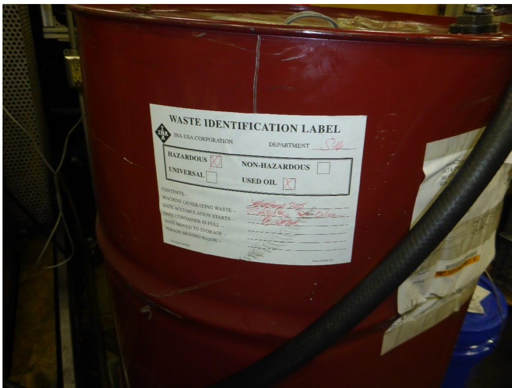
Photo 5: 55-gallon red metal drum in the Finger Follower Heat Treat Process Area. The waste identification label identifies the material as hazardous used oil, but Mr. Ratliff explained that the container of non-hazardous waste oil was mis-labeled.
