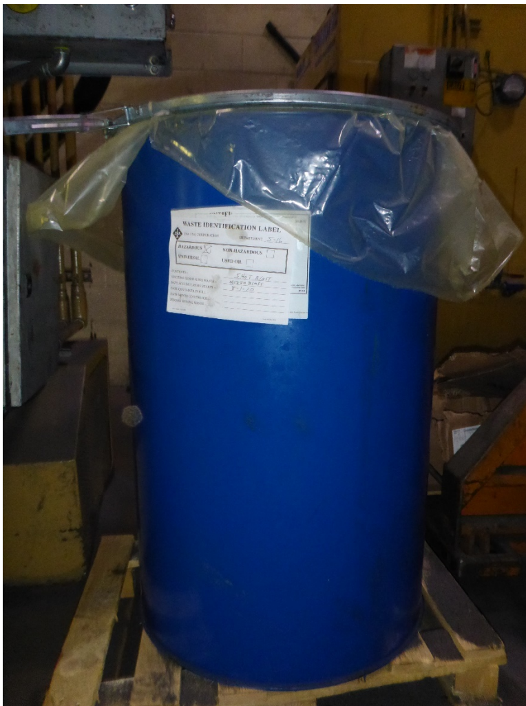
Photo 2: 55-gallon blue poly drum in the spent shot blast media SAA. The ring is not latched to secure the lid on top of the drum.
