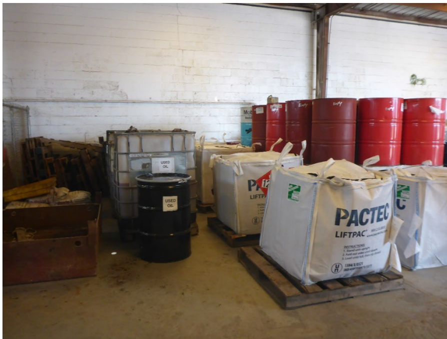
Photo 9: Rows of used oil totes, hazardous waste supersacks and empty drums without sufficient aisle spacing in the CAA warehouse.
