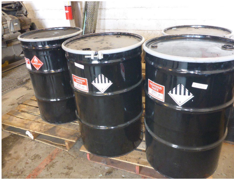
Photo 7: One 55-gallon drum labeled hazardous waste flammable liquid, and two 55-gallon drums labeled hazardous waste barium debris on wooden pallets in the CAA warehouse. The containers of hazardous waste barium debris were not marked to indicate that the contents are hazardous due to toxicity, and none of the drums were marked with the EPA hazardous waste codes.
