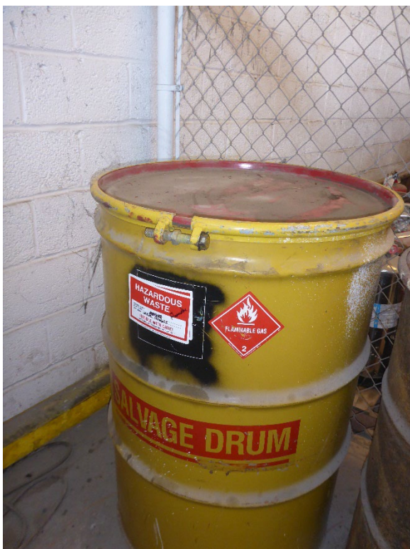
Photo 13: Empty salvage drum labeled hazardous waste aerosols located in the SAA at the far-left corner inside the CAA warehouse.
