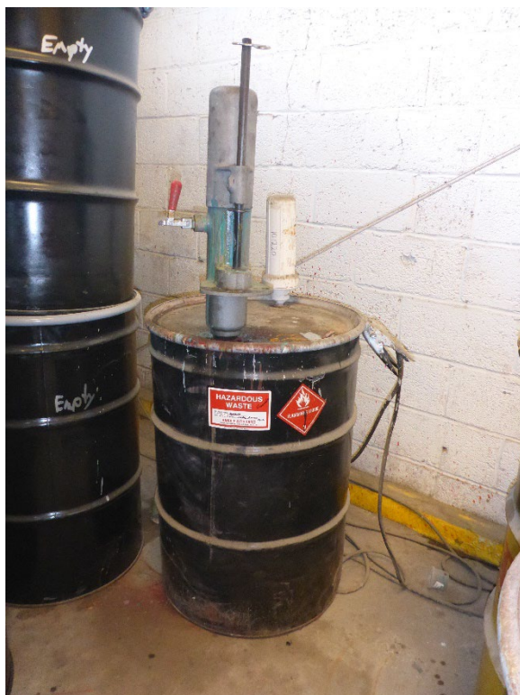
Photo 12: One 55-gallon drum equipped with a can puncturing device in the SAA located at the far-left corner inside the CAA warehouse.
