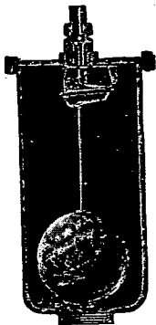
Trane Direct Return Trap in Section. Note that this Trap has no Stuffing Boxes, Outside Joints, or Weights
