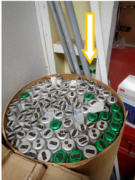
Picture 31 — Light Mechanical Shop Area— One (1) card board box was observed full of spent fluorescent lamps, even broken sections of spent fluorescent lamps. It was observed closed, not labeled as Universal Waste, not dated, was not under the operator’s control, and did not have a pictographic label and/or indication of the hazard. Additionally, three (3) spent fluorescent lamps were observed outside the round cardboard box.
