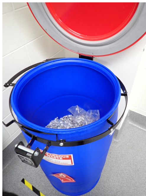
Picture 46 — Laboratory Area – Chemical Storage 26 Area— Here, one (1) 35-gallon blue plastic container with HPLC vials was observed closed, labeled as hazardous waste, and has a pictographic label available.
