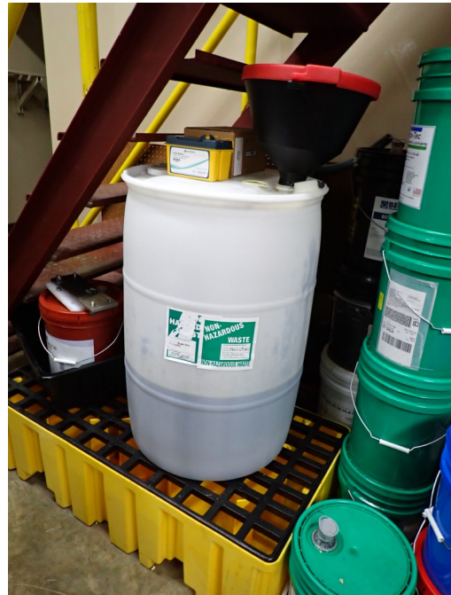
Picture 40 — Maintenance Shop Area— Here, one (1) 55-gallon white plastic container with Aceite usado was observed. It was closed, labeled as non-hazardous waste, and was placed above a secondary containment.
