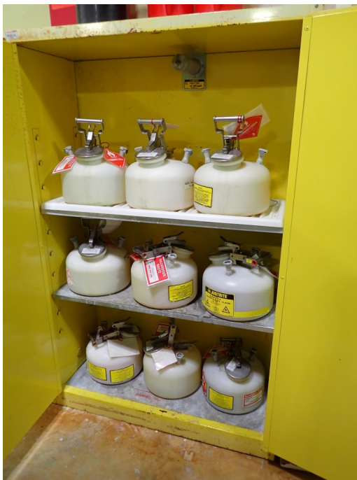
Picture 43 — Laboratory Area-Chemical Storage Q3 Area— Here, one (1) yellow shelf labeled as flammable and Full HPLC Safety Cans no halogenated waste was observed. Inside, the latter had nine (9) 2.5-gallon white plastic containers.
