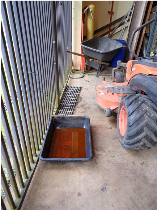
Picture 9 — Light Mechanical Shop Area— Just at the side of the tractor, an open container, not labeled and with an unknown content was observed.
