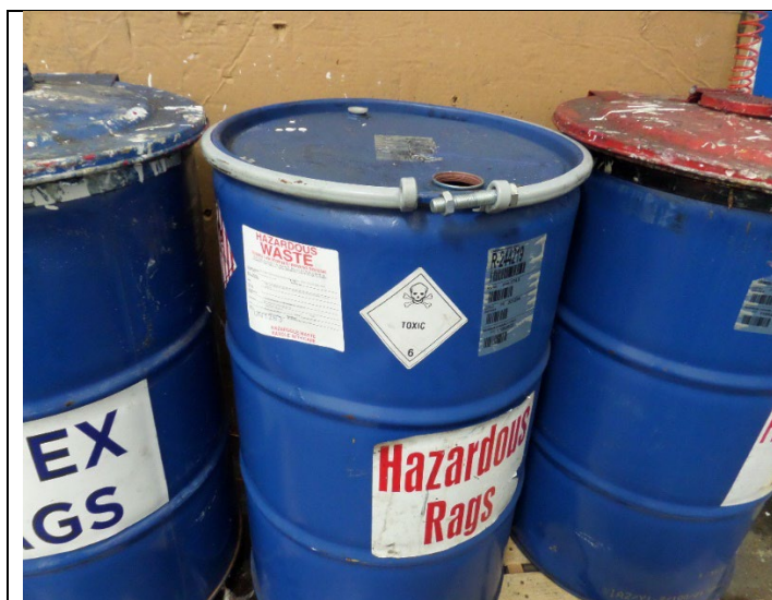
Repour Room. The top bung cap for the 55-gallon container of hazardous waste paint liquid was not kept closed and was not marked or labeled with a toxic hazard indicator. The facility closed and labeled the container. Photograph 15 taken at 1:05 p.m.
