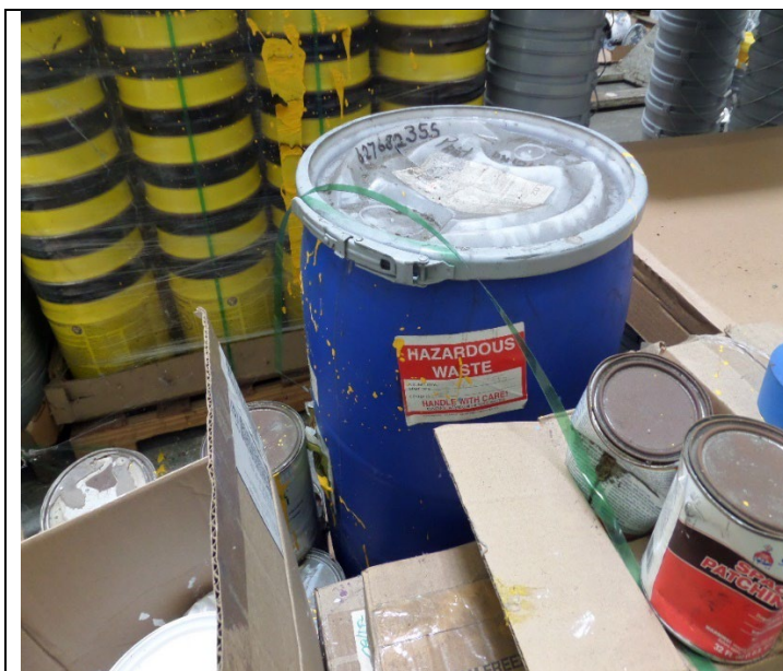
Repour Room. Observed a 30-gallon container accumulating waste paint mixed with absorbent labeled with the words “hazardous waste”. The waste appeared to have been generated by FedEx as clean-up material from a spill of the paint and returned to SWC. The container was not closed, was not marked with a date and not marked or labeled with a hazard indicator. Photograph 17 taken at 1:06 p.m.
