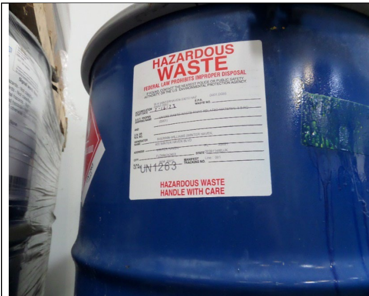
CAA. Observed a 55-gallon container accumulating hazardous waste (D001, D035), not marked or labeled with a toxic hazard indicator. Facility wrote toxic on the label. Photograph 3 taken at 11:38 a.m.
