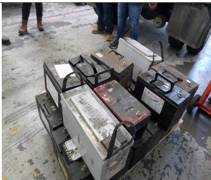
Trailer Maintenance Shop. Observed universal waste batteries not marked or labeled universal waste and not dated. Photograph 18 taken at 1:25 p.m.
