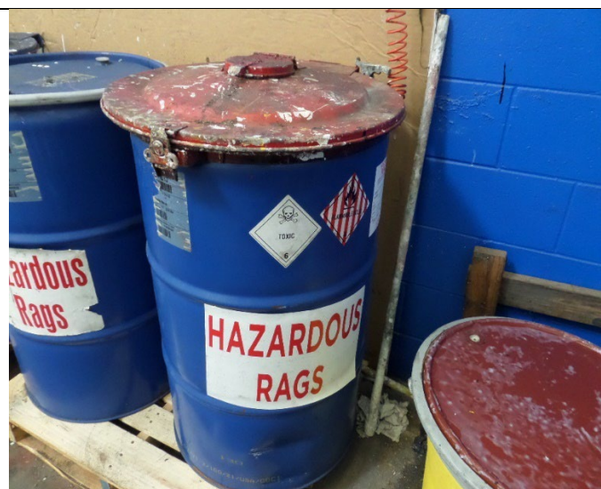
Repour Room. The 55-gallon container accumulating hazardous waste paint solid was not marked or labeled with a toxic hazard indicator. The facility labeled the container. Photograph 16 taken at 1:05 p.m.
