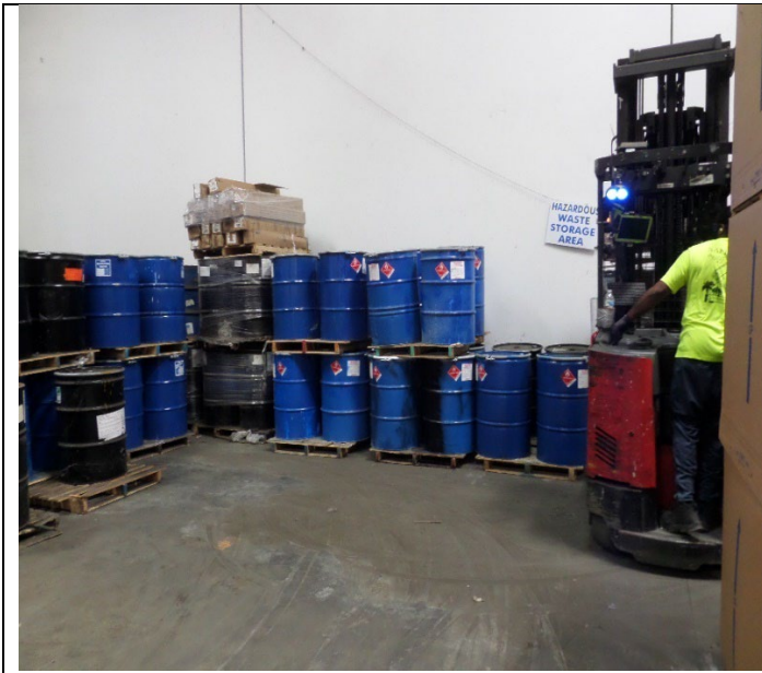
Central Accumulation Area (CAA). Observed needed aisle space. Facility rearranged containers and provided aisle space. Photograph 1 taken at 11:25 a.m.
