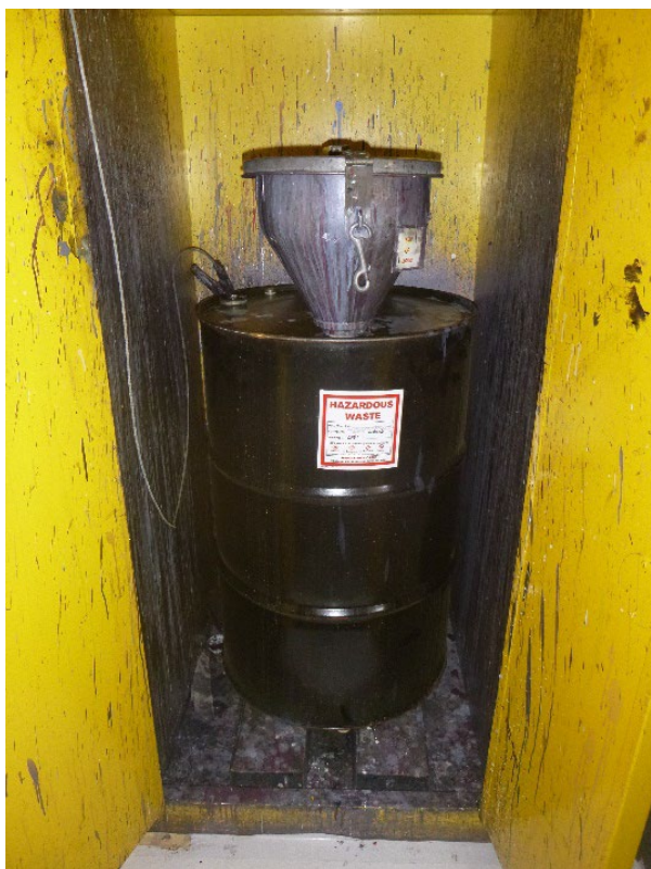
Photograph 1: SAA in Lab 1 without Indication of Hazard.
