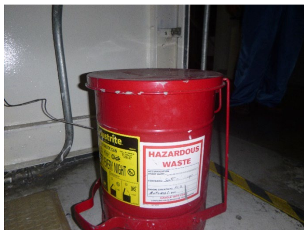
Photograph 9: SAA in Paint Line 2 without Indication of Hazard.
