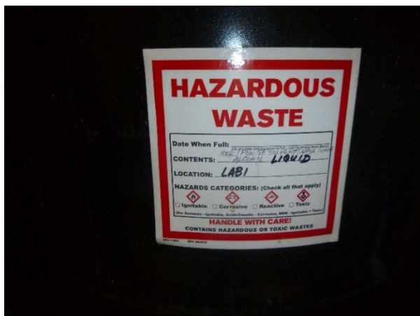
Photograph 2: SAA in Lab 1 without Indication of Hazard.
