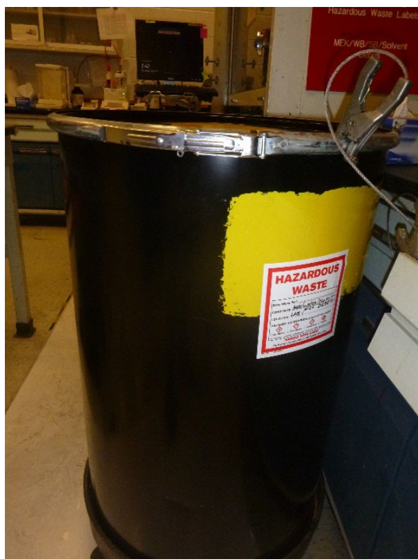
Photograph 8: SAA in Lab 1 without Indication of Hazard.
