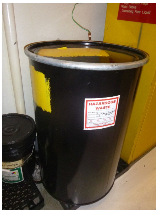
Photograph 4: SAA in Lab 1 without Indication of Hazard.
