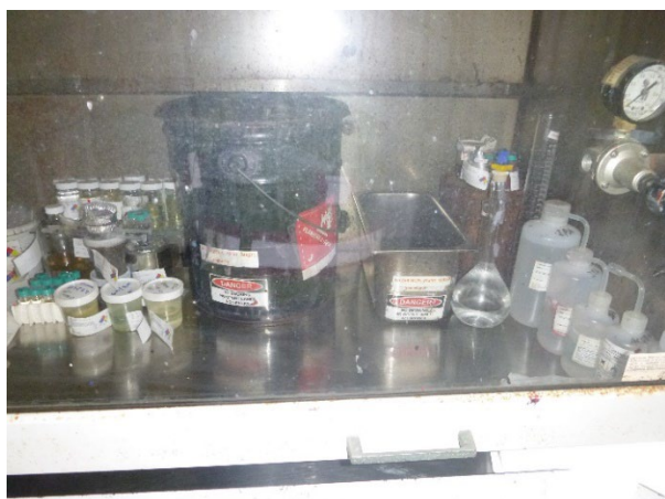
Photograph 7: SAA in Lab 1 without Indication of Hazard.
