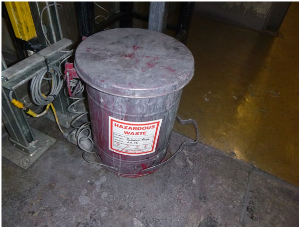
Photograph 10: SAA without Indication of Hazard.
