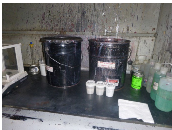
Photograph 6: SAA in Lab 1 without Indication of Hazard.
