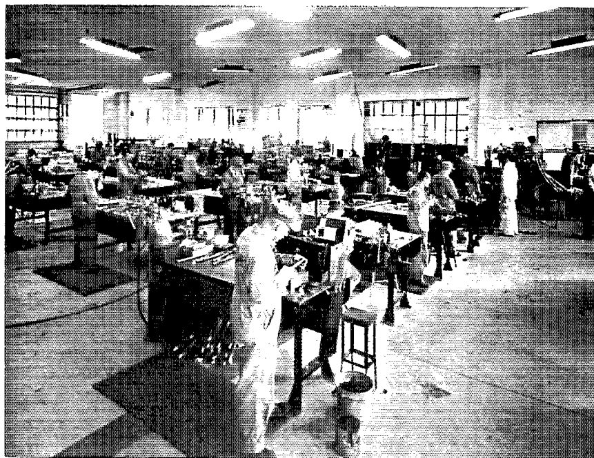
Mercury vapor long-tube lamps provide a satisfactory light for the exacting work of servicing planes of the United Air Lines.
