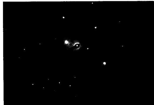
1/25/2013 HT 100KV TEM C1 60cm 1300866 Tremolite SAED; 0 angle near ZA
