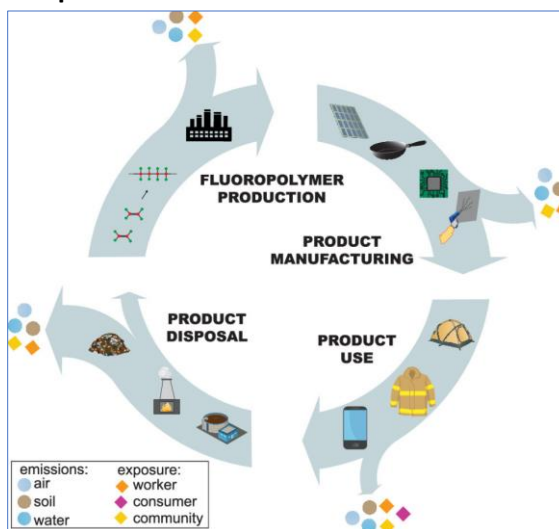
Figure 2: Conceptual diagram of PFAS emissions during fluoropolymer production, product manufacturing and disposal. Source: Lohman et al, 2022
