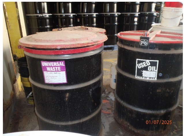
Picture 16 – HWSA used oil and universal waste containers
