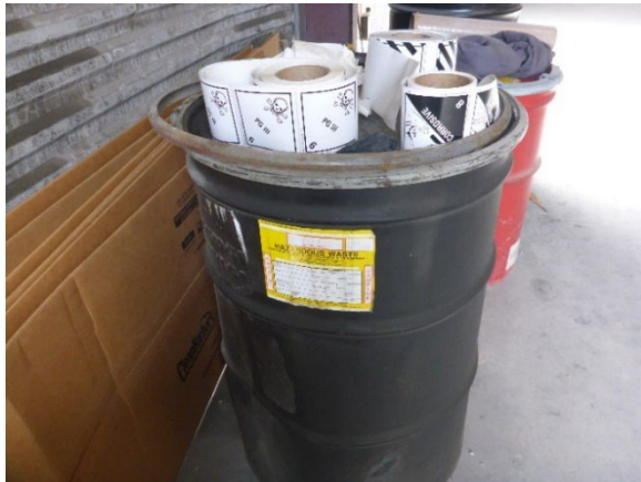
Photo 7 (Ten-day Warehouse SAA): Unsecured ring on 55-gallon drum of branch-generated debris. Drum is labeled hazardous waste, but not marked with an indication of the hazards of its contents.
