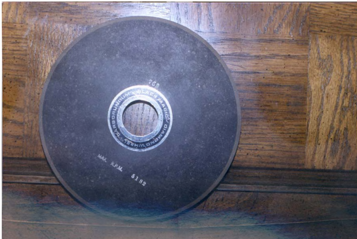
Figure A2. Carborundum Black Magic Diamond Wheel Grinding Wheel with black inner area
