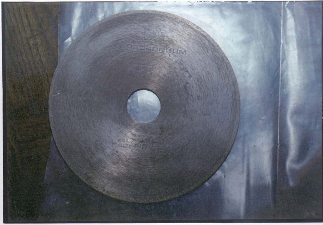
Figure A1. Carborundum Grinding Wheel with what appeared to be steel inner area.
