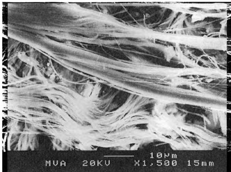
Figure B4. MVA0831-E0424: SE image of Post-it note adhesive surface showing chrysotile asbestos fibers. Magnification 1,500X.
