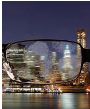
Figure 1: Antireflection coated lens with smudge: reflection increases and diffusion appears.
