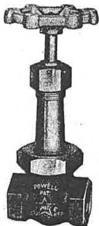
Fig. 376—200-pound Bronze Gate Valve with screwed ends, inside screw rising stem, union bonnet and renewable, wear-resisting "Powellium" nickel-bronze taper wedge solid disc in sizes 1/2" to 3/4", inclusive; taper wedge double disc in sizes 1" to 3", inclusive.
