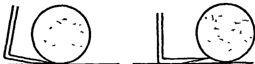
FIG 27-15—To pick up round objects, forks should be tilted (left), not used flat (right)
