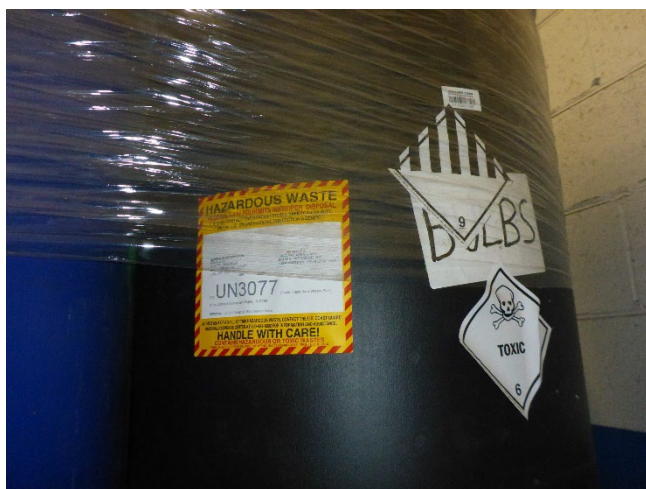
Photo 5 (P1010541.JPG): Hazardous waste container label, "crushed mercury containing bulbs" NHTC/Compatible Storage Area.
