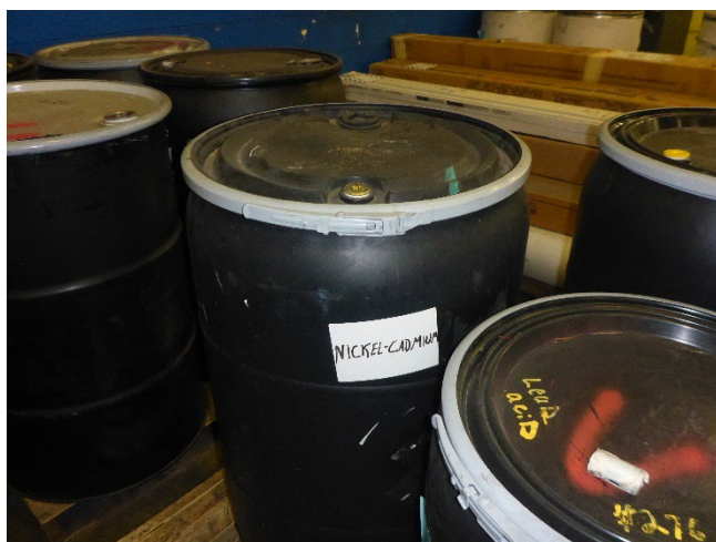
Photo 3 (P1010541.JPG): Universal waste battery container labeled as "Nickel-Cadmium" in the Universal Waste Area.
